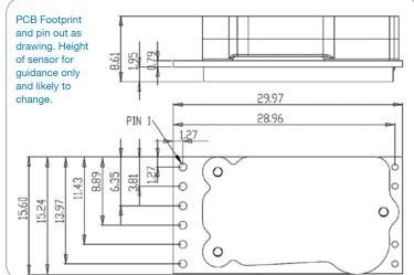
All dimensions in millimeters (mm)
