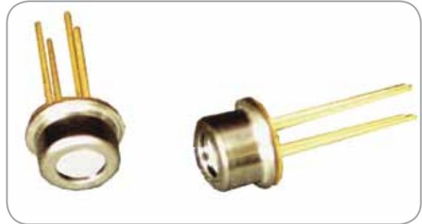
This thermopile sensor is used for non-contact surface temperature measuring. The ZTP-015 model consists of thermo-elements, flat IR filter, a thermistor for temperature compensation and a hermetically-sealed TO-41 (small-size) package.
