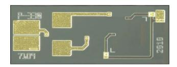
Amphenol Advanced Sensors' P330 piezoresistive pressure die offers the same superior stability and sensitivity as in larger chips, but in an extremely small footprint for invasive applications where small size is critical. It has excellent measurement accuracy, which is ideal for demanding applications with restricted dimensional profiles such as medical catheters and IC packages. NovaSensor's proprietary SenStable® process provides excellent long term stability and repeatability.
