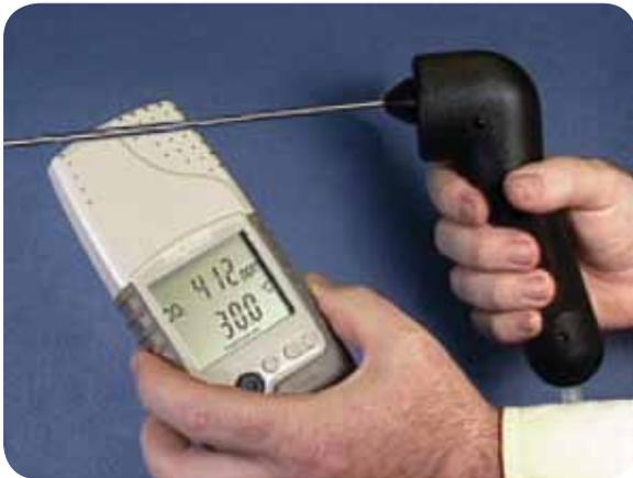
The Telaire Model 7001 hand held sensor can measure up to 10,000 ppm. The 7001 hand held monitor is compatible with any portable pump with an inlet and outlet that can deliver 80 to 100 cc/minute of air.
