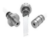
The piezoresistive sensor chip is housed in a fluid-filled cylindrical cavity and isolated from measured media by a stainless steel diaphragm and body. The modular design allows for variety of pressure port modules, which are hermetically welded to the die carrier. NPC Series Low and Medium Pressure Sensors
