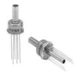
They are available in gauge, absolute and differential pressure versions in several pressure ranges from 10"  $H_2O$  to 100 psi (2.5 kPa to 700 kPa). The temperature compensation is provided by laser-trimmed resistors. The sensors are compatible with non-corrosive gases and dry air.
