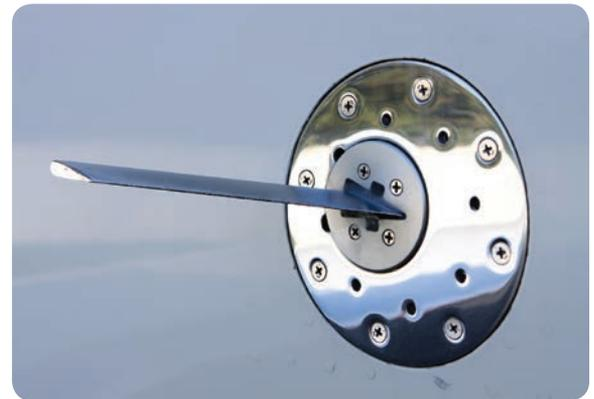
Angle of attack sensor on plane
