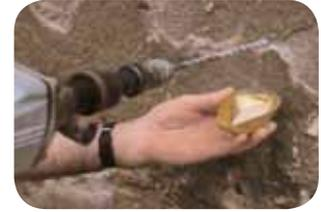
Moisture measurements are obtained by following a simple test procedure:
