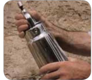
If the structure under investigation is contaminated with conductive hygroscopic salts, moisture meter readings may not truly reflect the moisture condition. Ambiguity that may be associated with interpreting moisture meter readings in contaminated material are reduced by also measuring the actual moisture content of wall or floor samples with the Speedy tester and by using a hygrometer to measure the material's equilibrium relative humidity (ERH).
