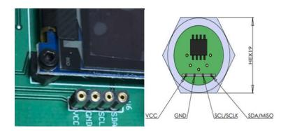
2. Connect Nova Sensor Evaluation board GND and VDD terminals to DC power supply and set power switch to ON position (~3-10mV voltage drop @Vin=3.3V expected).
